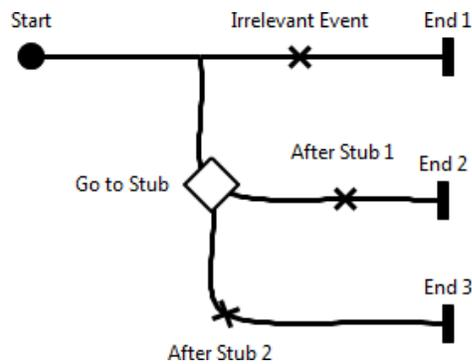
**Figure 19** A Pegasus can enter a stub
